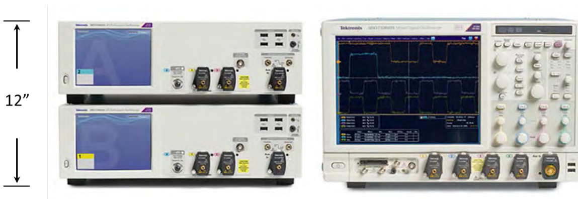
Figure 9: The compact size of the DPO70000SX enables efficient use of rack space for higher channel count. Shown here are two DPO70000SX units, with 4 channels at 33 GHz, next to an MSO73304DX with 2 channels at 33 GHz.
