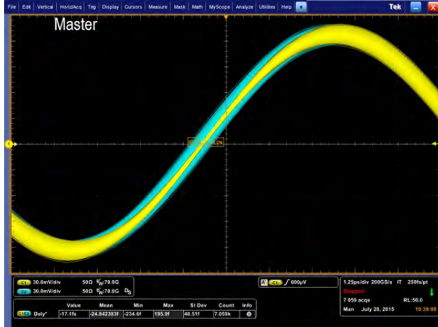
Figure 6: 65 GHz sinewave capture on two ATI channels illustrates inherently high channel-to-channel skew stability.
